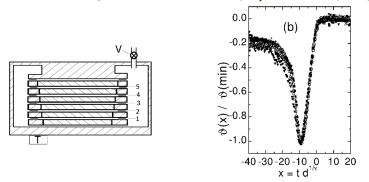
Setup: the thickness of adsorbed films is shifted from its expected value  $\Rightarrow$  evidence of the Casimir force.
